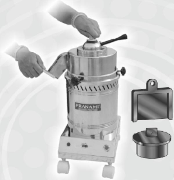
To avoid entering insects and dust. After finishing Grinding work fix round button and square cover at place of Hopper and Outlet bag respectively.
