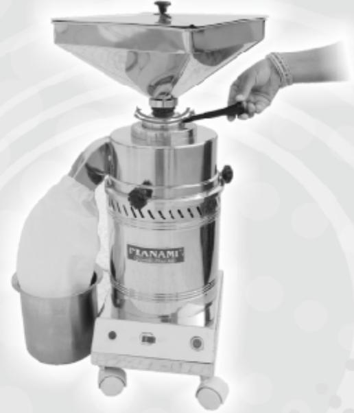
Turn regulator Handle clockwise for coarse grinding & anti-clockwise for Fine grinding.
